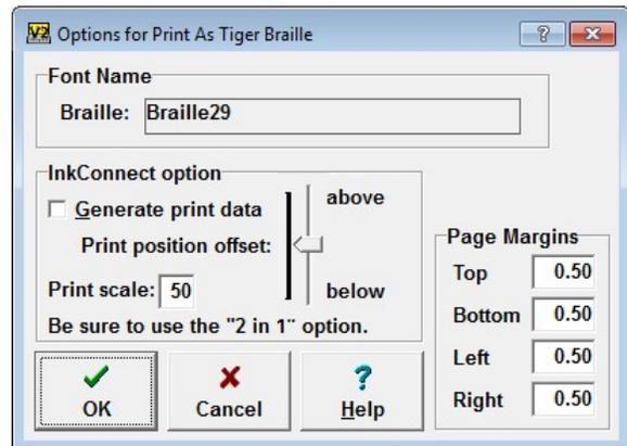
The Options dialog contains settings for Page Margins (in inches). The margin is the amount of space at the edge of the paper that comprises a border around the embossed area. The default values (half an inch) are generally appropriate. You can move the embossed area left or right by adjusting the values of the Left and Right margin amounts.
